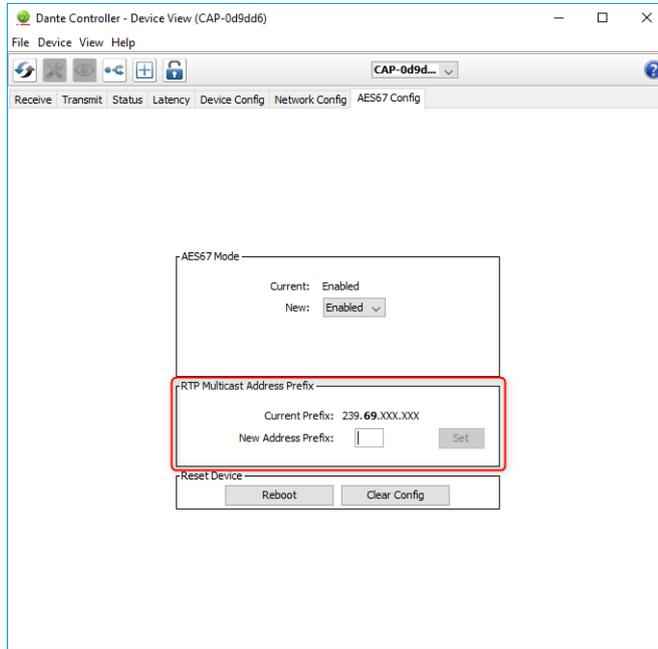
For AES67 mode, it is possible to modify the multicast address prefix via DANTE Controller software. In this mode, it is only possible to enter the second octet.
