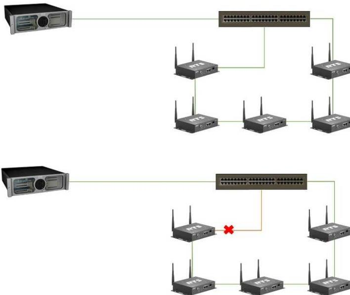
In this example, the devices are interconnected as a daisy chain loop. A daisy chain loop is easy and fast to install and can be used as an ad-hoc solution. In case of cable or device failure between devices, the communication path continues via the other end. If the device contains an Ethernet port(s) and fiber optic port(s) both marked as OMNEO, a combination of Ethernet and fiber can be used to extend the distance between the switch or router and first connected devices of the chain.
