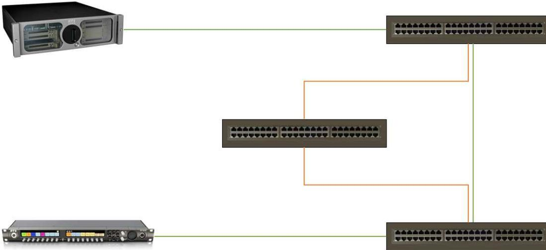
In this example, the direct connection between two switches has failed. As RSTP is active, the routes are known and another route is taken for communication between the devices. Also, there is only one back-up connection, but with RSTP there can be multiple routes available not just one or two.
