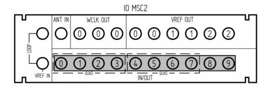
Synchronization can either be derived from internal clock, GPS input, or external video reference (BB or Tri-Level). GMC supports up to 256 simultaneous PTP agents.
