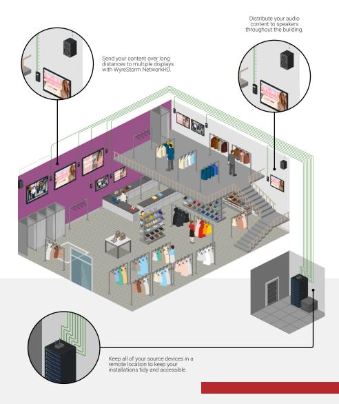
WyreStorm's NetworkHD uses AV over IP technology. AV over IP (Audio Visual over Internet Protocol) uses a set of rules to send AV signals over a Network. With this technology, the sky's the limit when it comes to the number of sources and displays you can use. Many NetworkHD models allow you to switch between sources with virtually no lagging, making them perfect for showing the big game, special events or even digital signage across any hospitality environment.
