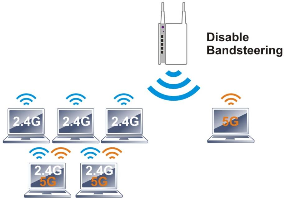
If dual-band is detected, the AP will let the wireless client connect to less congested wireless LAN, such as 5GHz to prevent network congestion.
