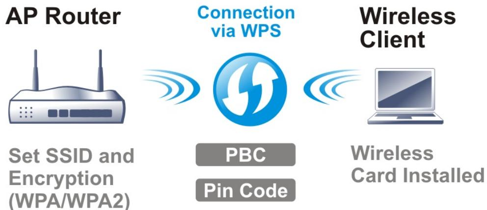
It is the simplest way to build a connection between wireless network clients and VigorAP 903. Users do not need to select any encryption mode and type any long encryption passphrase to set up a wireless client every time. He/she only needs to press a button on wireless client, and WPS will connect for client and VigorAP 903 automatically.
