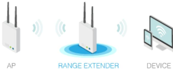
The access point can act as a wireless repeater; it can be Station and AP at the same time. It can use the Station function to connect to a root AP and use the AP function to serve all wireless stations within its coverage.
