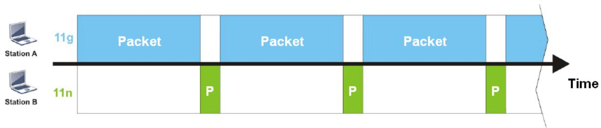
To improve this problem, Airtime Fairness is added for VigorAP 903. Airtime Fairness function tries to assign similar airtime to each station (A/B) by controlling TX traffic. In the following figure, Station B(11n) has a higher probability to send data packets than Station A(11g). In this way, Station B(fast rate) gets fair airtime and its speed is not limited by Station A(slow rate).
