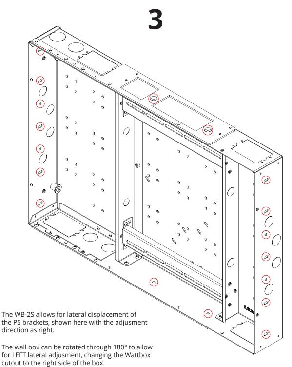
• The WB-2S should be inserted into the wall cut out from the front, then secured to the surrounding studs using the 40mm pozi head wood screws provided through the Ø6.5mm [0.25"] fixing holes circled below.
