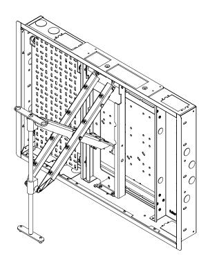
The larger shift side can be to the left or right depending on wall box orientation. Rotate the wall box 180° to determine shift direction.
