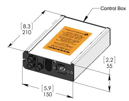
Note: TTR Mechanism cables will run from the mechanism to the Control Box.
