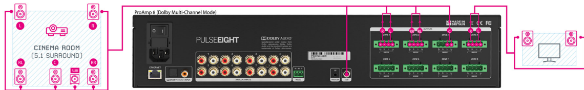
Figure 1: Connecting the audio output for 3 Zone Dolby Mode
