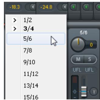
**Trim Gains.** After a click on the **T** symbol one channel's faders are all synchronized. Instead of changing only a single routing the fader affects all the channel's active routings. For a better overview the faders currently not visible are indicated by orange triangles beside the fader path. When moving the fader the triangles also move to a new position, equalling the fader's new settings.
