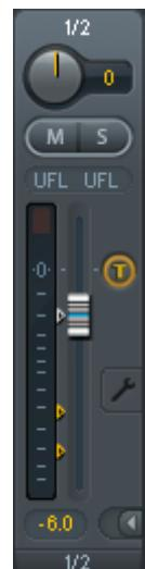
In View Options / Show the function Trim Gains can be globally switched on and off for all channels. This global Trim mode is recommended when using TotalMix FX as live mixing desk.
