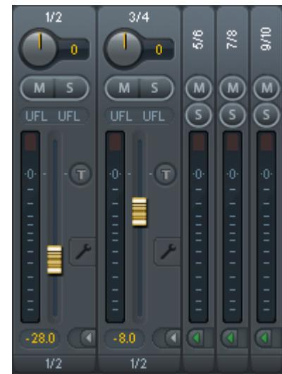
A Shift-click on a fader adds the fader to the **temporary fader group**. All faders now marked yellow are ganged, and move simultaneously in a relative way. The temporary fader group is deleted by a click on the F symbol in the upper right of the window.
