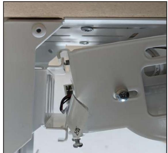
**2** Once Shade is hooked onto the **Sub Bracket**, lower the shade so that the locking bolts drop behind lower return on **Mount Platform**. Both locking screws can tightened to lock shade in place.
