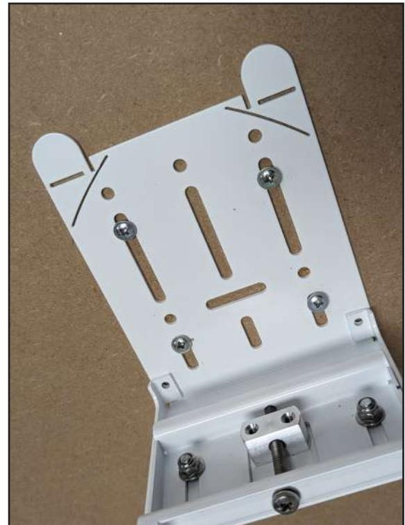
The fixings can be loosened and each **Sub Bracket** position adjusted slightly forwards or back using the slots, if their position needs to be fine tuned.
