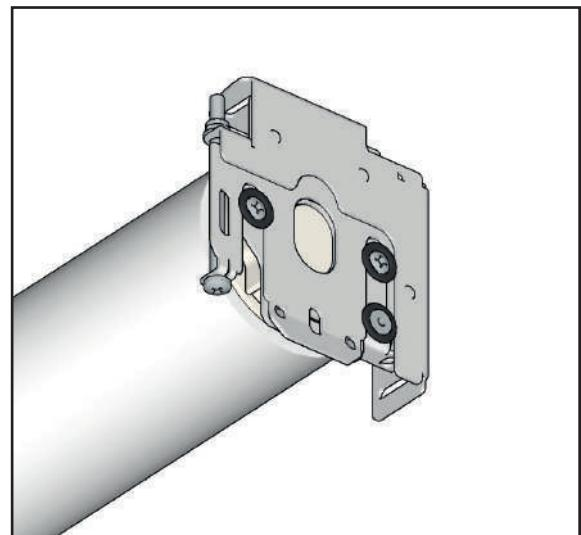
**2** Each **Sub Bracket** has two large open slots that the **Plastic Guide Bushes** on the **Mount Bracket** will locate into while the shade is being lifted up into the **Sub Brackets**.
