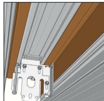
For additional security, the **Sub Brackets** can be secured into the Bracket Mount Rail by tightening the pre-installed grub/set screws or by putting suitable fixings (not supplied) through the slots in the top return on the bracket into the aluminium of the Bracket Mount Rail.
