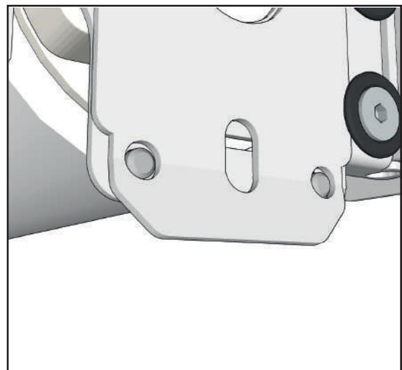
**4** Once the Mount Bracket has engaged onto these set screws, one of the supplied **M5 x 6mm Pozi Thread Forming Bolts** can be installed into the folded return on the bottom of each of the **Mount Brackets** to lock it securely to the **Sub Bracket**.
