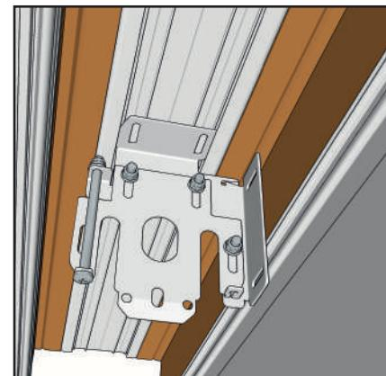
Each **Sub Bracket** can be repositioned by twisting it clockwise to unlock, then sliding it along the Bracket Mount Rail to the desired position before twisting back to lock into place.
