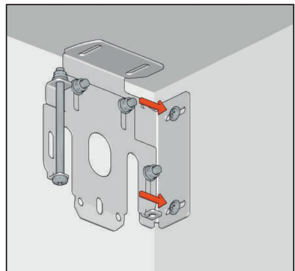
The fixings can be loosened and each **Sub Bracket** position adjusted slightly left or right using the slots, if their position needs to be fine tuned.
