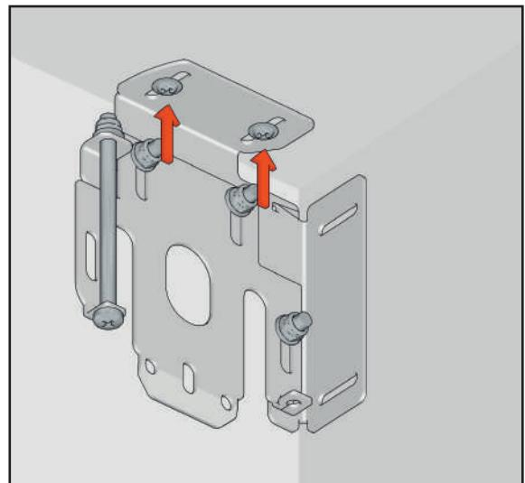
The fixings can be loosened and each **Sub Bracket** position adjusted slightly forwards or back using the slots, if their position needs to be fine tuned.
