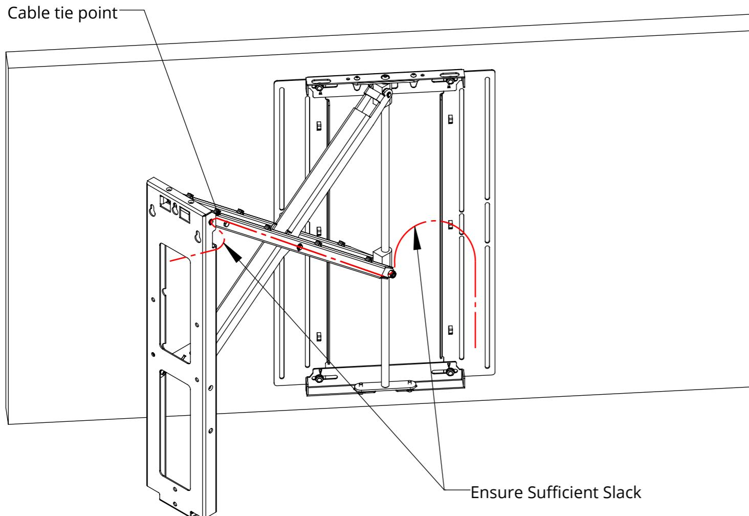
Wall sockets should be ideally placed as shown outside of the bracket footprint to maximise space for cable routing
