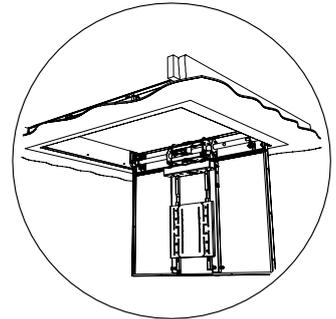
5. Loosen Clamp Bolts on both sides of tray
