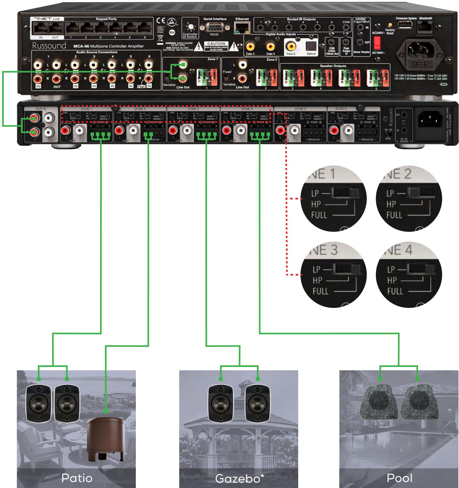
\*The D-Series amps are stable to 4 ohms, so you can add 2 pairs of speakers where needed.
