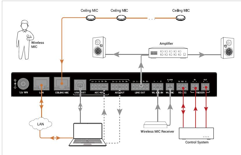
**Note:** After the device is connected to a computer, it can be detected by the system and specific applications as a speaker and a microphone in the name of **COM-MIC-HUB**.
