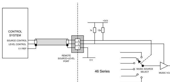
**NOTE:** If the control voltage source is not isolated from the power earth, there is a small risk of creating a 'ground loop' by linking the mixer technical ground (0 V) to the ground (0 V) of the equipment supplying the control voltages. To minimise this risk, we suggest that all pieces of equipment be in close proximity, and supplied from the same power outlet.
