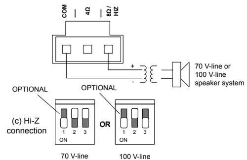
When driving 70/100 V-line loudspeaker systems there is a risk of transformer core saturation at high levels and low frequencies, which can produce distortion. To prevent this, the mixer-amplifier's output stages are provided with a 65 Hz high-pass filter, which may be enabled by setting **SPEAKER CONFIGURATION** switch SW1 to ON (switch down).
