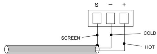
12 V phantom power is available at both mic inputs, and is activated by setting internal jumpers J9 (Mic Input 1) and/or J1 (Mic Input 2) to the ON position. See page 27 for locations of internal jumpers. Care should be taken to ensure that phantom power is activated only when the microphone connected to the input requires it – i.e., a capacitor or electret type; other types of microphones (such as dynamic) may be damaged if a DC voltage is applied to them.
