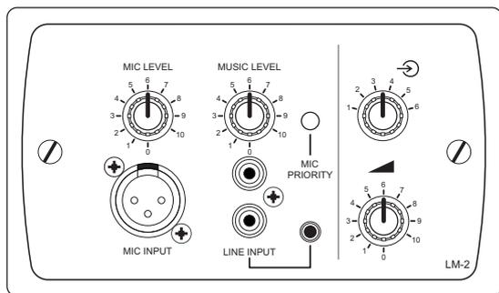
LM-2 mic/line input module, with music source and level controls
